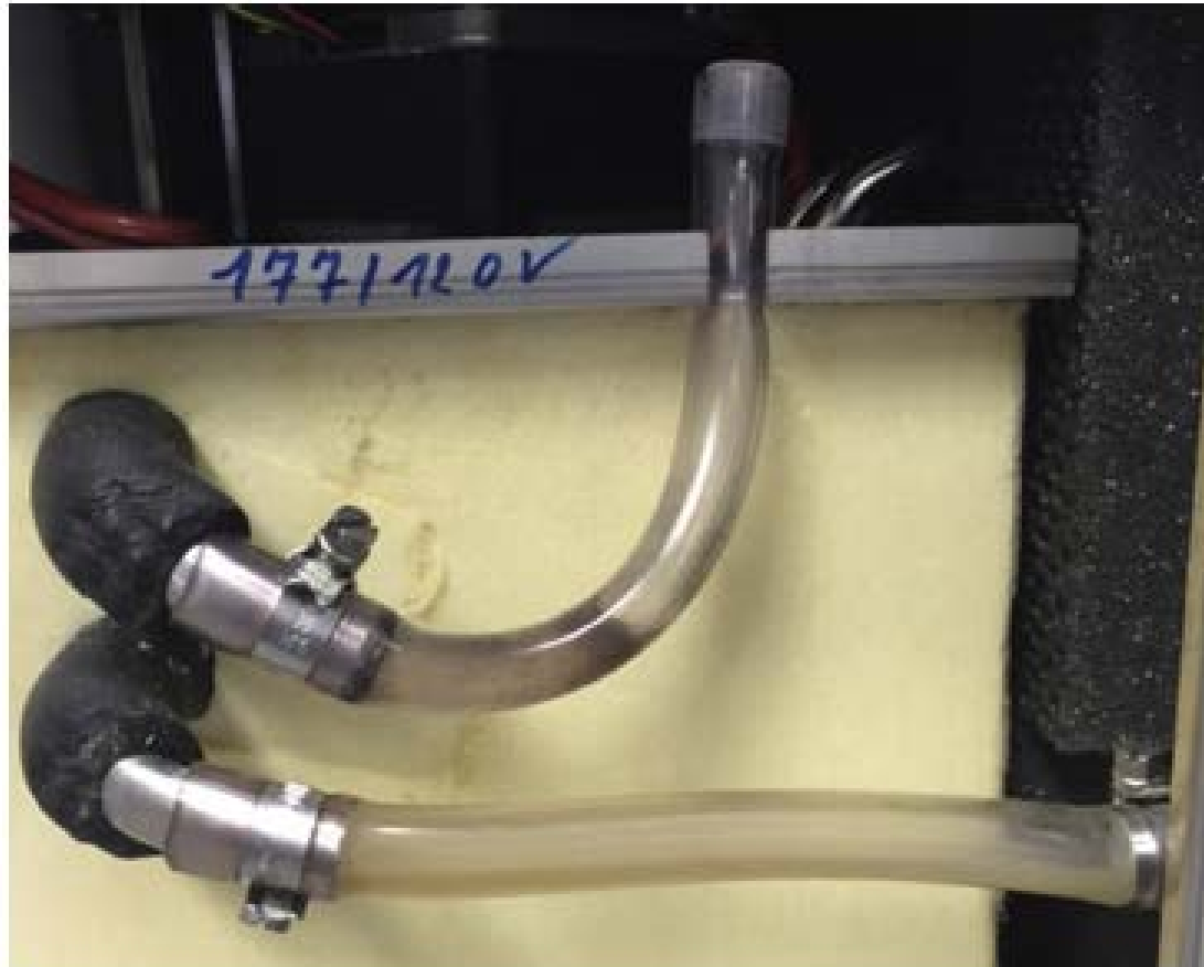
Fig 2. Inside a heater-cooler device (LivaNova/Sorin Stöckert 3T, Munich, Germany) demonstrating biofilm formation in the plastic tubing (ie, discoloration) despite cleaning per manufacturer recommendations.
